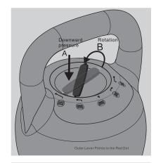
3. While adjusting the weights, must make sure the Adjustment Saucer will bounce and stay in lock position. Must make sure the Outer Lever points to the dots on top of the number.
