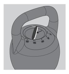
2. In order to re-select the weights, the Kettlebell must return to its base. After finish with the exercise, must return the Kettlebell to the base and select the heaviest weight to lock the Kettlebell.
