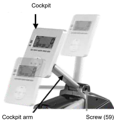
To be able to read the cockpit of your rowing machine optimally or to adjust the cockpit position for different body sizes, the inclination of the cockpit arm and the cockpit are stepless adjustable by hand. Check regularly the tightness of screws (59) which fixes the cockpit arm. If necessary, use the Allen key M8
