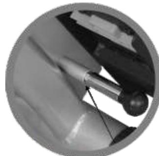
Safety Pin (34B) in locked position
