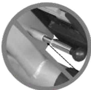
Safety Pin (34B) in unlocked position
